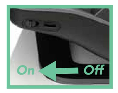
Slide the On/Off switch on the back of the left module away from the USB port to power it up. Then power-up right module next. Note: For best syncing, always power the left module first.
