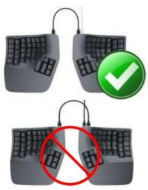
Connect the two key modules using the Link Cable. The Link Cable must be connected to the left module's right port and the right module's left port.
