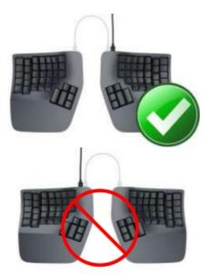
Then, connect the right module to the PC using the Main Cable
