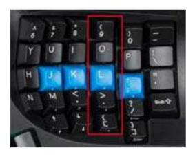
Keys are arranged in vertical columns (Fig 4) to reflect the natural motions of your fingers, and the keywells are sculpted and concave to fit the varying lengths of your fingers. This shortens reach and reduces the time to learn touch typing for new typists.
