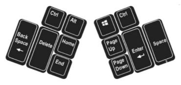
Activating Mac Mode changes the modifier thumb keys, as shown in Fig 15. The Mac "command" action is the "Windows" action in a Windows operating system. The Mac "option" action is the same as Alt in Windows. Two additional keys change in Mac Mode:
