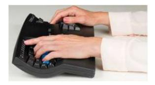
Cherry ML low-force, tactile mechanical kekeyitches are used in the function key row (Fig 7) for a great typing fe, consistency, and long life. These keycaps are laser legends. As on all Contoured keyboards, the function keys are positioned closer to the alphanumeric keys to reduce the reach.
