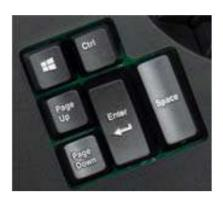
The left and right thumb clusters (Fig 3) feature commonly used keys such as Enter, Space, Backspace, and Delete. Modifier keys such as Control and Alt on the PC and Command and alAltption on Macs have also been relocated to the thumb clusters. Windows users will appreciate a Windows key in the right thumb cluster. By moving these commonly used keys to the thumbs, the Advantage2 redistributes the workload from your relatively weaker and overused little fingers to your stronger thumbs.
