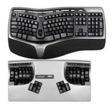
By removing the traditional numeric 10-key keypad and embedding it into the right alphanumeric well in the Keypad layer, Kinesis was able to reduce the overall width of the Advantage2, making it much smaller (16 5/8 x 8 1/8 x 3 inches) than a traditional keyboard (Fig 8). This smaller footprint allows closer placement of any pointing device, reducing over-reach issues.
