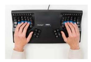
Separating alphanumeric keys into left and right key wells (Fig 2) reduces strain and stretching by positioning the arms approximately at shoulder width, with the wrists straight. This design reduces abduction and ulnar deviation, which are harmful postures that can lead to repetitive strain injuries such as carpal tunnel syndrome and tendonitis.
