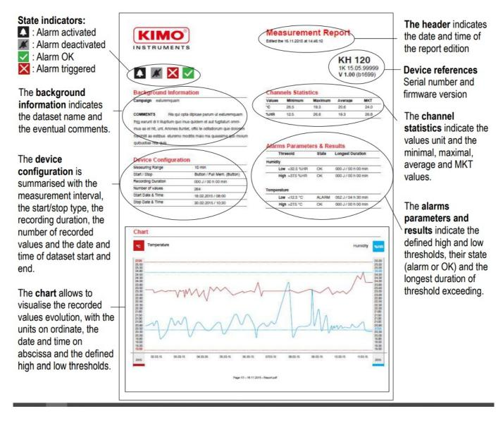
You can print it or export it in PDF format to integrate it easily to your documents. **Configuration, datalogger download and data processing with the KILOG software** Please see the **KILOG** software user manual: "**KILOG-classes-50-120-220-320**".
