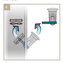
5. Remove the grommet in the opposite lock hole by pushing it out from the inside of the cover
