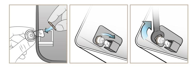
1. Insert the Left Push Button tab through the cover opening, and thread Lock Nut over tab
