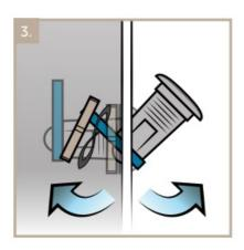
4. Remove the lock nut and wave washer, then remove the remaining lock assembly by maneuvering it through the hole.
