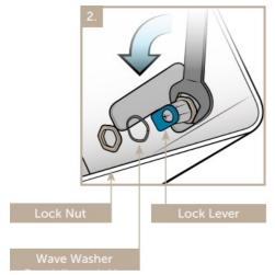
3. Maneuver the lock nut around the lock lever by pulling the entire lock assembly out and pivoting to work it through the hole.
