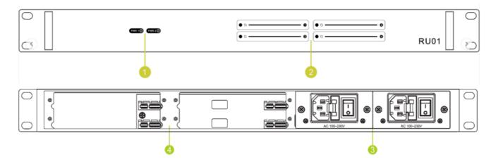
PWR1 and PWR2 respectively correspond to two power status indicators, and four card indicators display four card working states.
