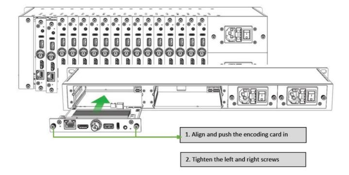
By designing the RE-3 in a card form factor, you can easily install and adjust its integration with the Cradle series chassis. This design takes into account users' professional needs, allowing for a more flexible deployment and management of the equipment. Moreover, this integrated design can reduce the need for extensive device connections and wiring, simplifying the overall system configuration and maintenance.
