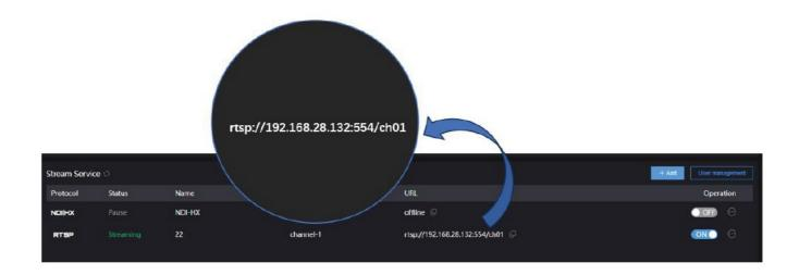
Click to copy this address, you can check the encoded video stream by pulling the stream through VLC.
