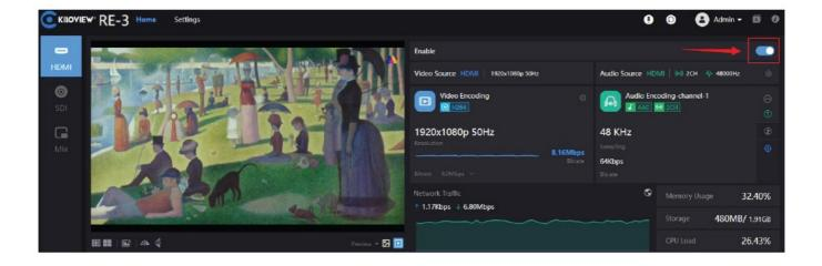
If you need to switch between HDMI and SDI video sources, you just need to click on the leftmost navigation bar on the web page. Clicking on "SDI" selects SDI video source encoding and clicking on "Mix" enters the mixed encoding mode.
