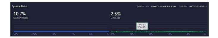
When the system memory and CPU are too high, please confirm whether the performance of the NDI Core device is insufficient due to a large number of transmissions. You may need to update your hardware system. The timeline below shows the memory and CPU usage in the past time, and the current time is 0s.
