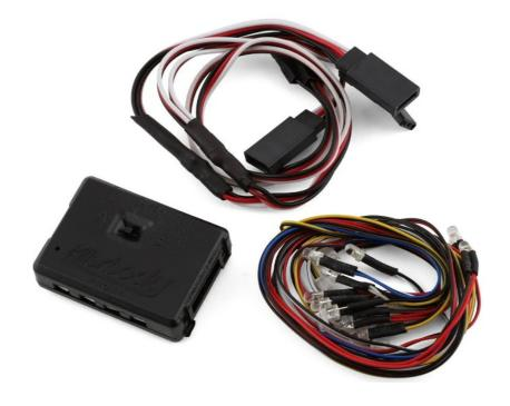
lights set, please pre-check proper fixure location before using 3M double-sided tape to fix it. We suggest to fix the LED lights set at the nearest area to the signal receiver which on the bottom of the chassis.
