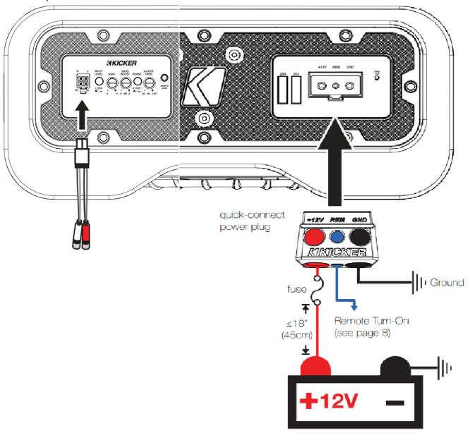
If needed, cut off the RCA connections to use hilevel input, or use the KICKER KISL Speaker-RCA Converter. quick-connect wiring harness audio inputs:
