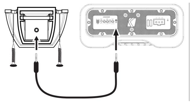
Connect the cable to the remote and the Remote Bass connection on the amplifier
