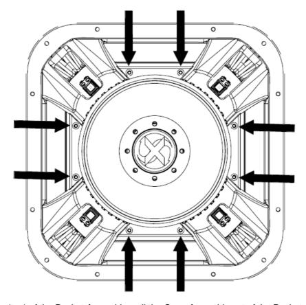
• From the cone side (top) of the Basket Assembly, pull the Cone Assembly out of the Basket Assembly.
