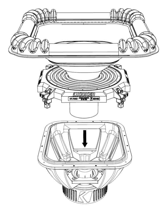
Secure the Spider to the Basket Assembly using the eight M5x0.8x16mm bolts. Loosely start all bolts before tightening. Torque the bolts to 20in-lbs in the sequence shown below.
