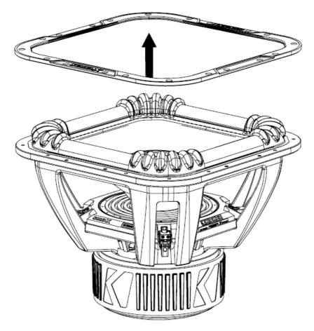
• From the magnet side (bottom) of the Basket Assembly, use a 4mm Allen Wrench to remove the eight M5x0.8x16mm bolts securing the Spider to the Basket Assembly.
