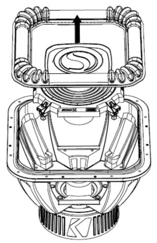
• Clean and remove all debris from the Voice Coil Gap.
