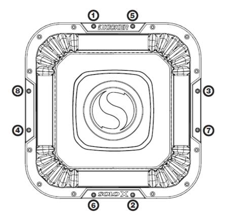
Remove the Voice Coil Alignment Pins from the motor.
