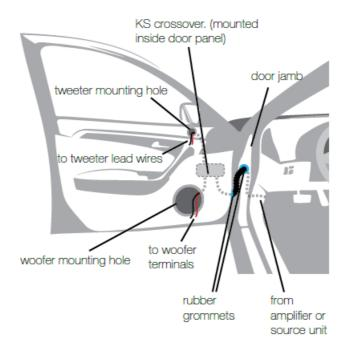
If factory speaker wiring is not available in your desired location, it may be necessary to run speaker wire through the door jamb. The speaker wire should be kept away from sharp edges and avoid the possibility of getting pinched by the door. An existing grommet in the door jamb is the ideal place to run the speaker wire. If the factory hole and grommet do not exist
