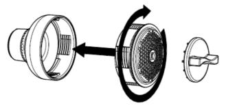
Thread the tweeter wire through the lower tweeter post and insert the tweeter assembly to the tweeter post until it clicks into place
