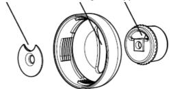
Attach the tweeter to the tweeter housing using the included tweeter tool
