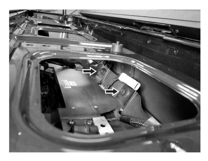
9. Install the amplifier onto the amplifier bracket with the supplied amplifier screws (short screws x 4).
