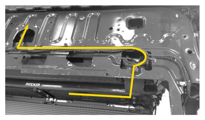
15. Disconnect the trailer connector and install the T-harness between the trailer connector and the factory harness.
