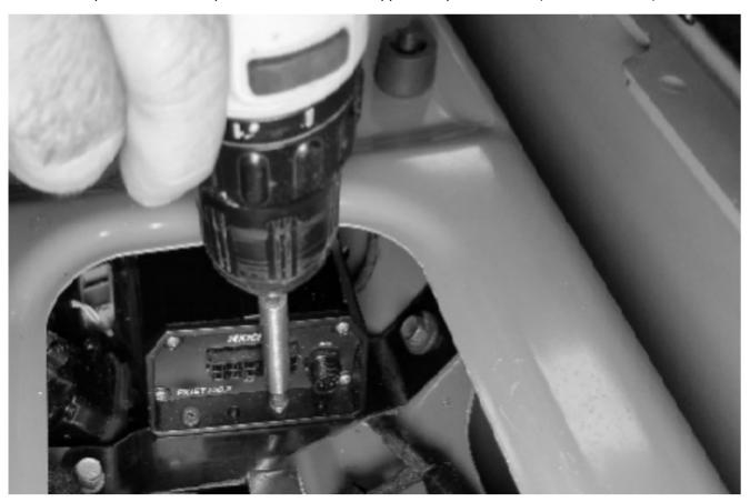
10. Connect the amplifier harness to the amplifier and the four-pin connector to the tilt switch attached to the amplifier bracket.
