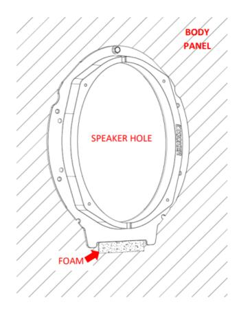
5. A back gasket/spacer is included to improve fitment. It may be necessary to space the speaker motor further way from accessories (windows tracks, lock actuators, etc.) in some applications. If necessary, use the back gasket/spacer.
