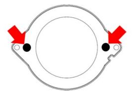
3. Route KCS270 wires and motor through the flange. NOTE: Place flange over terminals first, then locate speaker in flange.
