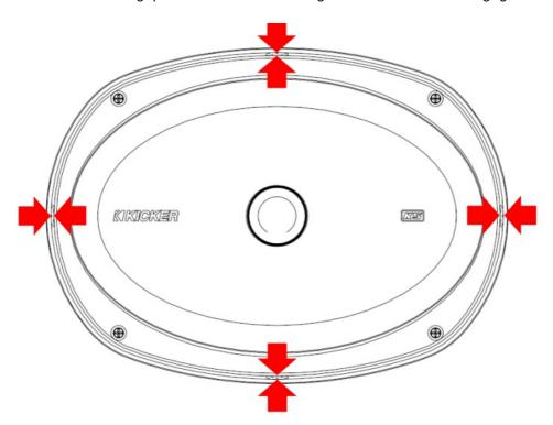
5. Carefully insert grille into the gap in the bezel.
