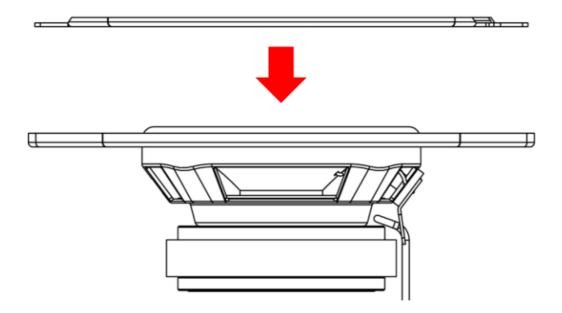
5. Rotate speaker to desired orientation in the flange.
