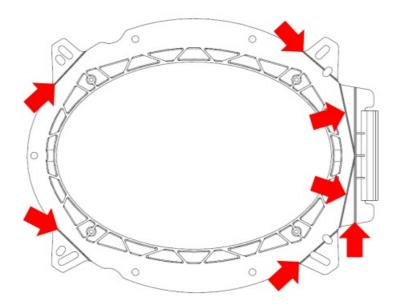
3. For some applications the adapter clips to the mounting panel on one side. It may be necessary use the foam damper to tighten the fitment of the clip-on side of the adapter.
