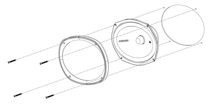
4. Apply the black adhesive into the gap of the bezel where the grille's tabs insert and engage the bezel.
