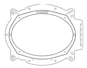
2. Using side cutters remove any tabs that may impede installation of adapter or reassembly of factory components. Cutting locations are molded into the backside of the adapter.
