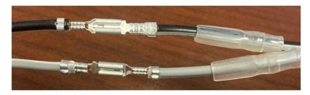
2. Slide the clear cover over the terminals to prevent a short circuit.
