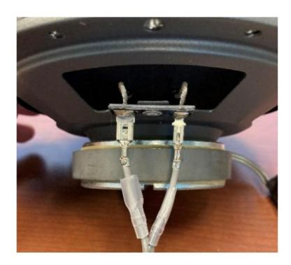
2. Slide the clear cover over the terminals to prevent a short circuit.
