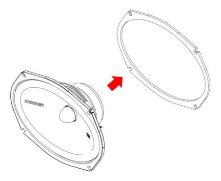
6. Fasten the mid-bass woofer to the adapter using the supplied screws.
