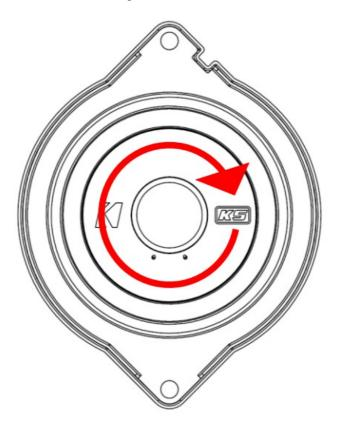
6. Fasten speaker to mounting location using the factory hardware or supplied screws.
