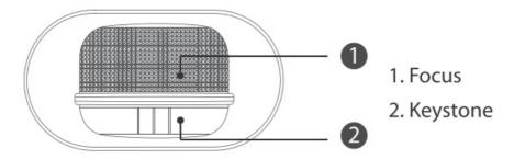
Some projectors focus by rotating the lens, and the trapezoidal correction is located on the back of the machine.
