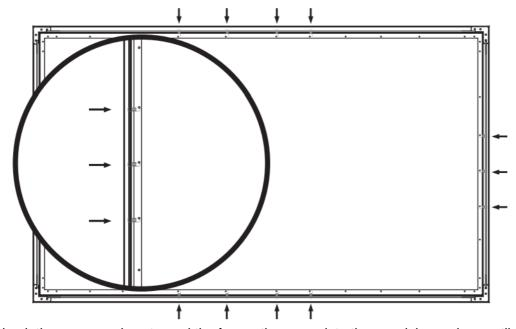
4. Continue to hook the corner springs toward the frame, then complete the remaining springs until the screen is
