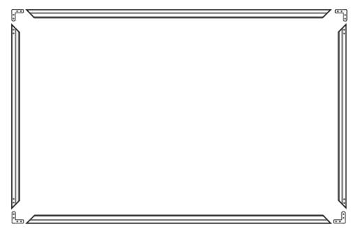
2. For this step we recommend washing your hands, avoid touching the white side of the screen, and use a clean cloth sheet underneath. Roll out the projector screen with the black side facing up, and slide the fiberglass rods into the four side pockets of the screen.
