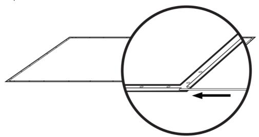
3. Place the screen with the white side facing down on top of the facing down frame to hook the springs. Start by placing the spring in the middle part of the screen (3-4 on each side), pulling them toward the frame.
