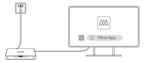
3. Using the Mind App, update the BIOS and EC. After the update is completed, unplug the power supply and HDMI cable from Mind
