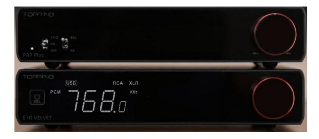
You can control the volume on PA7 and PA7 Plus, or set to bypass the volume control of PA7 and PA7 Plus, then you can use a better pre-amplifier for volume control.
