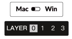
• If your system toggle is switched to Windows, then the layer 2 will be activated. Remember that if you are using it in Windows mode, please make changes to the layer 2 instead of the top layer (the layer 0). This is a common mistake people are making.
