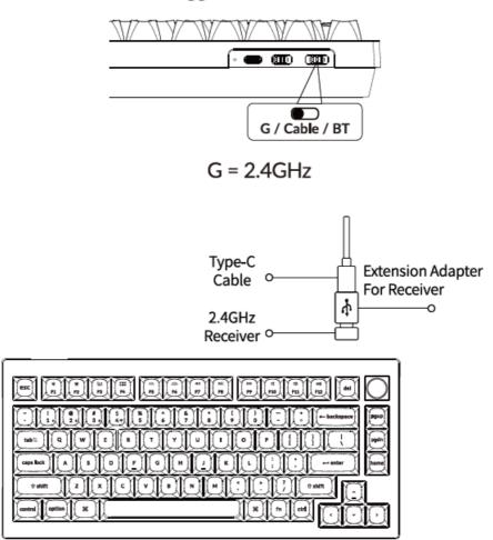
**Note**: For the best wireless experience, we recommend using the extension adapter for receiver and putting the 2.4GHz receiver somewhere on your desk close to your keyboard for a low rate of latency and fewer signal interferences
