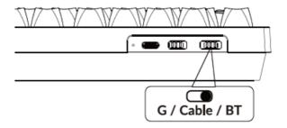
Press Fn + 1 (for 4 seconds) and pair with device named V1 Max.
