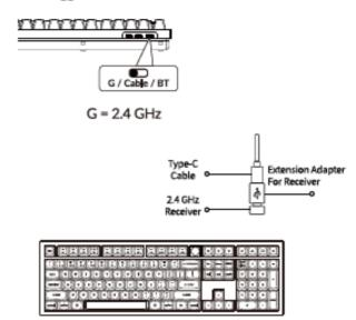
Note: For the best wireless experience, we recommend using the extension adapter for receiver and putting the 2.4 GHz receiver somewhere on your desk close to your keyboard for a low rate of latency and fewer signal interferences.
