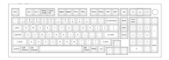
LAYER 1: This layer will be activated when your keyboard's system toggle is switched to Mac and press the fn/MO(1) key.
