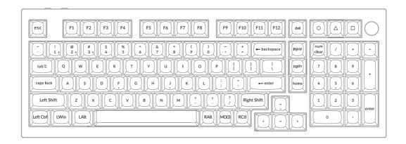
LAYER 3: This layer will be activated when your keyboard's system toggle is switched to Windows and press the fn/MO(3) key.
