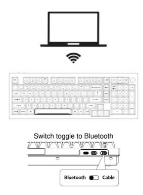
Press fn + 1 (for 4 seconds) and pair with device named Keychron Q5 Pro.
