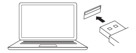
• Connect the 2.4 GHz receiver to the device USB port.
