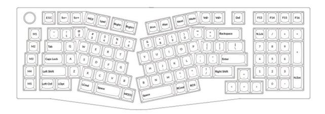
LAYER 1: This layer will be activated when your keyboard's system toggle is switched to Mac and press the fn/MO(I) key.
