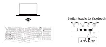
Press fn + 1 (for 4 seconds) and pair with device named Keychron Q13 Max
