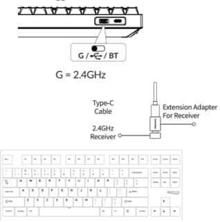
**Note:** For the best wireless experience, we recommend using the extension adapter for receiver and putting the 2.4GHz receiver somewhere on your desk close to your keyboard for a low rate of latency and fewer signal interferences.
