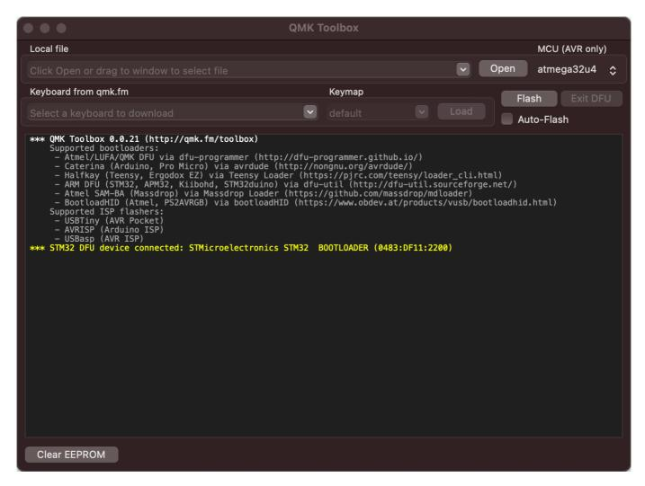
6. Click open and choose the Keychron Q2 firmware. Click the Flash button. It will start flashing. (Note: Do NOT unplug the power cable while it's flashing.)
