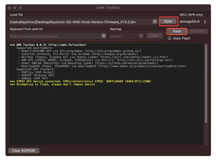
7. Wait a few seconds and when you see the content below, it means the keyboard has flashed successfully factory reset.
