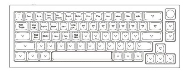
**LAYER 4**: This layer will be activated when you press the fn2/M0(4) key.
