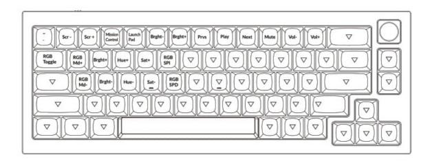
LAYER 3: This layer will be activated when your keyboard's system toggle is switched to Windows and press the fn1/M0(3) key.
