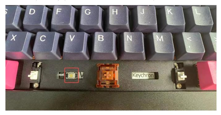
5. Press down and hold the reset button, then plug in the power cable. The keyboard will enter into DFU mode. Then, the QMK Toolbox will display in yellow words "\*\*\*DFU device connected".
