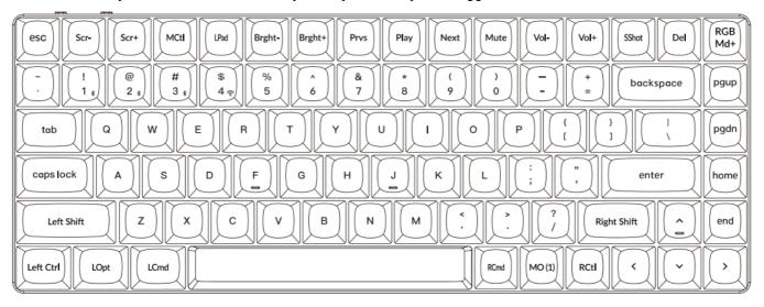
**LAYER 1**: This layer will be activated when your keyboard's system toggle is switched to Mac and press the fn/M0(1) key.
