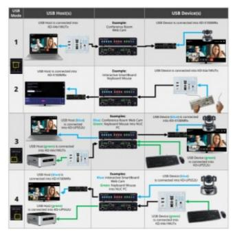
\*Use USB hub for multiple USB devices into KD-X4x1WUTx
