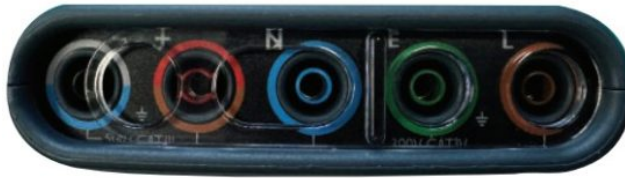
Fig.2 Interlock in position for RCD & Loop testing
