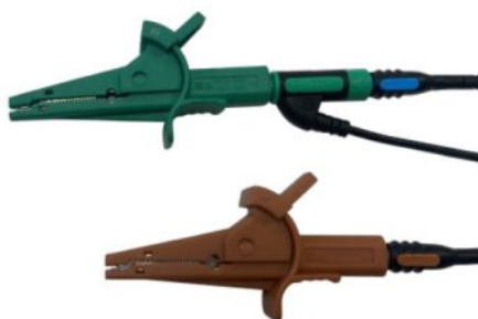
Fig 4. Crocodile clips in 2 wire testing configuration
