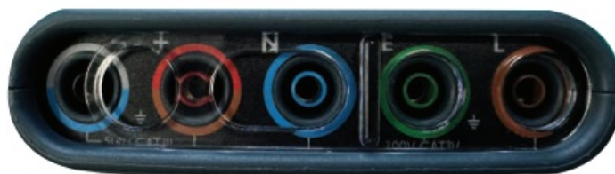
Fig.2 Interlock in position for RCD & Loop testing
