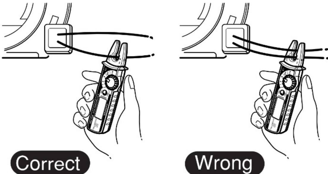
Place the center of the measured conductor lower than the triangle mark indicated on the fork shaped sensor. (shaded part in the figure)
