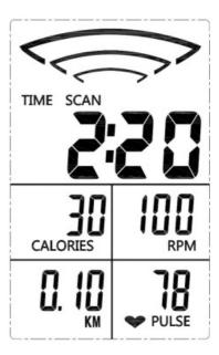
During exercise, in SCAN state, SPEED and RPM switch every 5 seconds. Press the MODE key to switch the display and turn on or off the SCAN function. Process: SCAN  $\rightarrow$  (RPM or SPEED)  $\rightarrow$  (SPEED or RPM)  $\rightarrow$  SCAN
