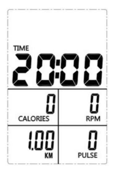
On the DISTANCE GOAL screen the user shall be able to choose the desired distance for their workout. The user shall be able to enter a distance from 1.00 to 99.50 kilometers. The user can adjust the value up or down by using the PLUS and MINUS buttons respectively. Each press of either the PLUS or MINUS button shall change the current displayed value by 0.50. The PLUS button shall be used to increase the length and the MINUS button shall be used to decrease the length.
