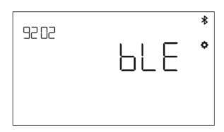
Once a connection has been made to a BT HR strap, the console shall also be able to connect to a smartphone app simultaneously. The behavior described above applies. Note that a connection must be made to a heart rate strap before establishing a connection to a smartphone if you want to connect to both simultaneously.
