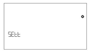
To enter SETTINGS MODE press WORKOUT button and navigate with +/- to SETTINGS MODE and confirm with WORKOUT button.
