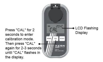
While "CAL" is flashing in the display, press "CAL" again to start the calibration. When the calibration is finished, the display shows "End".
