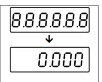
Should the balance not display exactly zero despite empty weighing pan, press the will be set to zero after a short standby time.
