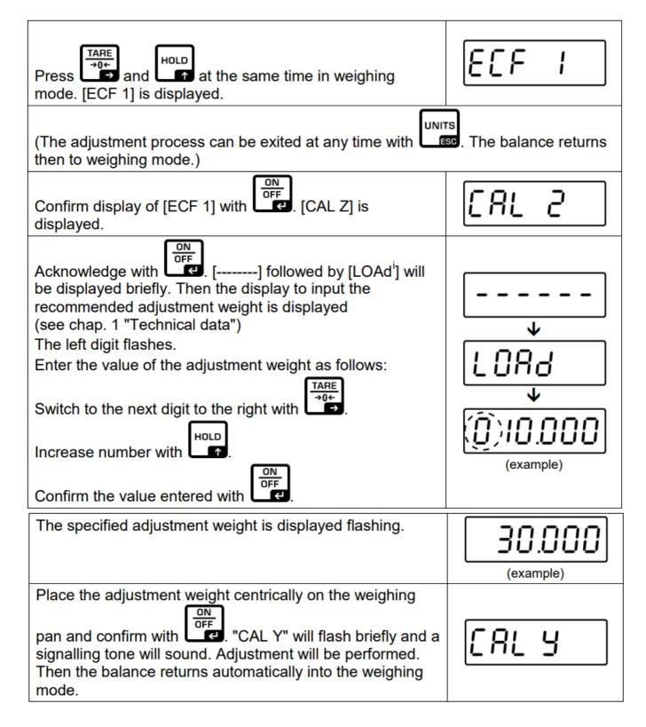
An error message will be displayed in the event of an adjustment error or incorrect adjustment weight. Remove the adjustment weight and repeat the adjustment process.
