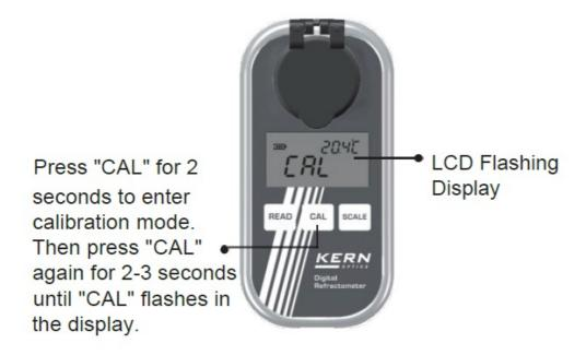
While "CAL" is flashing in the display, press "CAL" again to start the calibration. When the calibration is finished, the display shows "End". After approx. 10 seconds, the device automati- cally returns to normal mode.
