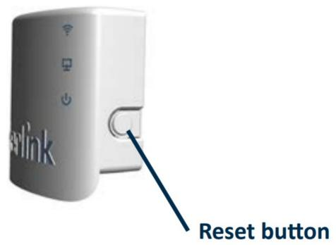
Short press the "Reset" button (<5s) to generate a software reset of the product. See LEDs behaviors in the dedicated LEDs table.
