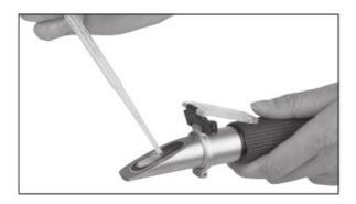
Your refractometer has an automatic temperature compensation (ATC). The reference temperature is 20°C (68°F). **Explanation of results**
