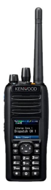
The NX-5000 Series is a digital radio system that offers three different protocols for the enterprise and public safety use: NXDN, DMR, and P25.
