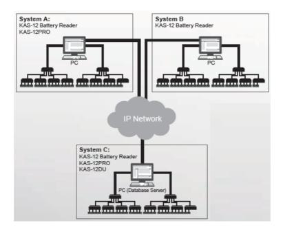
Create Battery Reader Management System over IP networking by installing KAS-12DU Battery Reader Database Utility on a server and authenticating the KAS-12PRO Software Upgrade License for the system. Monitoring is enabled only on a system with KAS-12PRO authentication.
