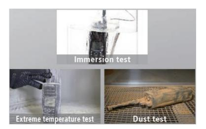
During the development stage, NX-5000 Series radios go through a number of stringent tests to make sure they can withstand harsh usage. In addition to MIL-STD-810 C/D/E/F/G environmental standards, NX-5000 portable radios comply with IP67/68 immersion standards, offering max. 2 hour protection at a depth of 1 meter\*. The rugged mobile radios comply with IP54/55\*\* dust/water ingress protection standards.
