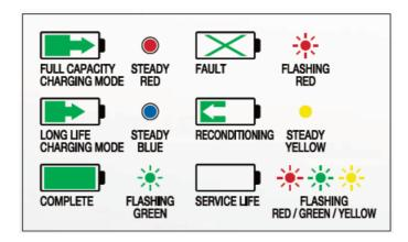
Battery conditions are displayed in color illuminated indicators on the charger, which are also displayed on a connected PC with the same color scheme. Color-coordinated patterns provide users with at-a-glance information for comprehensive battery management.
