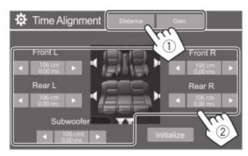
3. Touch [Gain] (1), and then adjust the sound level of each speaker (2).
