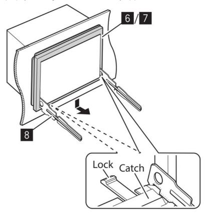
2. When the lower level is removed, remove from the upper two catches of the trim plate (6/7).
