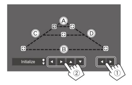
Make sure that A and B are horizontally parallel, and that C and D are the same length.
