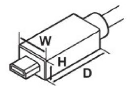
W: 11.1 mm or less H: 7.7 mm or less D: 21.5 mm or less
