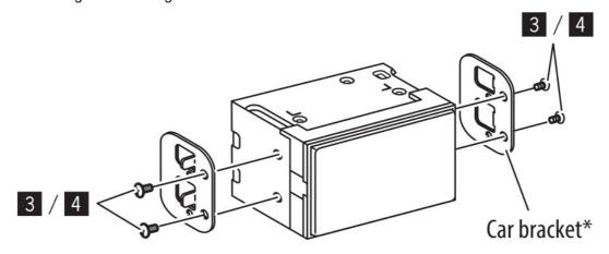
**Note:** Select the appropriate screws (supplied) for the mounting bracket.
