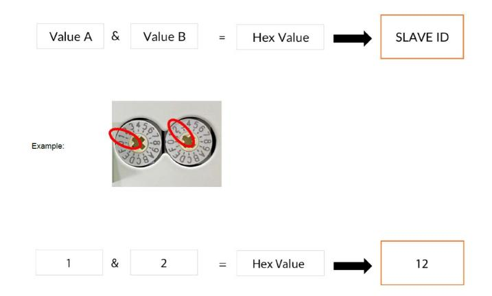
**Important Note**: The combination of 0 and 0 or F and F are not functional. Please ensure these configurations are avoided to maintain proper operations.
