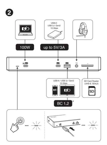
USB Battery Charging 1.2-Compliant device (up to 5V/2.4A for Apple Device)
