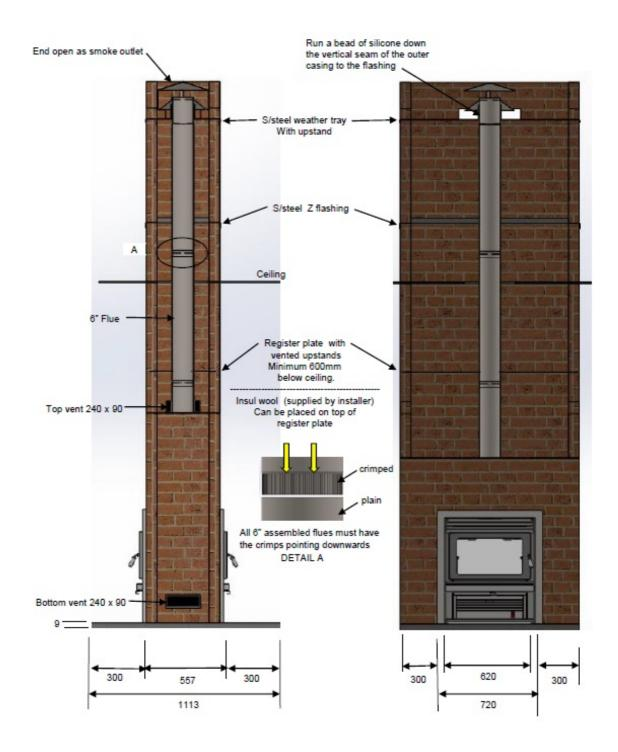
NB The opening on each side and top should allow for a gap (minimum 20mm) from fireplace body to allow for heat expansion. (i.e. for a gap of 20mm the opening would be 665 wide x 745 high)
