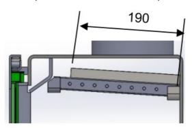
3. PLACE BAFFLE PLATES AS FAR BACK AS POSSIBLE, 190 MM FROM FRONT TO BACK.
