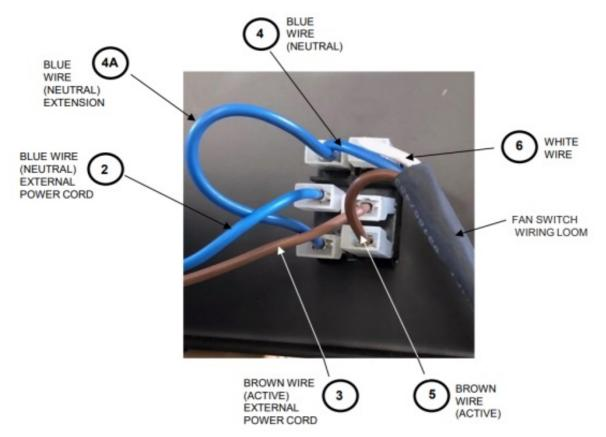
6. WHEN ALL THE CONNECTORS ARE IN PLACE, TURN POWER ON AND TEST, IF THE FAN TURNS ON, THEN THE ASSEMBLY IS COMPLETE.
