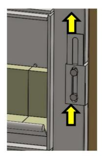
4. PUSH THE PACKER FROM THE BOTTOM EDGE OF THE ADJUSTMENT ANGLE UNTIL FULLY REMOVED. ONLY TAKE OUT WHAT IS NECESSARY. RE-POSITION THE ADJUSTMENT ANGLE AT THE MARKERS AND TIGHTEN.
