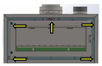
2. THREAD ONE SCREW AND ONE WASHER (SUPPLIED) TO EVERY NUT SERT SHOWN. MAKE SURE THE WASHER IS AS CLOSE TO THE SCREW HEAD AS POSSIBLE. LEAVE ENOUGH GAP FOR THE FASCIA TO SLIDE BETWEEN THE BOX AND THE WASHER.
