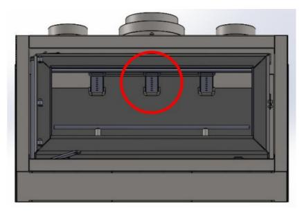
5. RE- PLACE MIDDLE AIR TUBE BACK INTO POSITION ( NB. MAKE SURE OPEN END OF AIR TUBE IS PLACED INTO REAR OPENING. CLOSED END TOWARDS DOOR. FAILURE TO INSTALL AIR TUBES CORRECTLY WILL VOID WARRANTY.)
