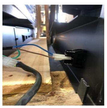
5. PLUG IN THE WIRE CONNECTORS TO THE FAN SWITCH, REFER TO DIAGRAM BELOW FOR PLACEMENT (CONNECTED BROWN AND BLUE WIRE SHOWN FROM EXTERNAL POWER CORD)
