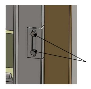
3. LOOSEN THE 2 BOLTS AS REQUIRED. DO NOT UNSCREW THE BOLTS ALL THE WAY OUT.
