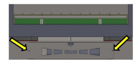
1. REMOVE 2 SCREWS HOLDING THE FAN CASSETTE IN PLACE
