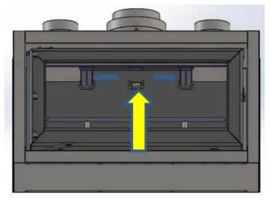
2. PLACE ALL 4 BAFFLE PLATES ABOVE AIR TUBES BOTH SIDES CLOSEST TO THE FIRE BOX WALL AS SHOWN ( 2 LEFT AND 2 RIGHT)
