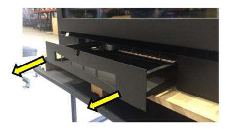
3. PULL THE FAN CASSETTE AWAY FROM THE APPLIANCE, ABOUT HALF WAY OUT, THEN GENTLY PULL THE FAN WIRE LOOMS BACK INTO THE FAN CASSETTE.
