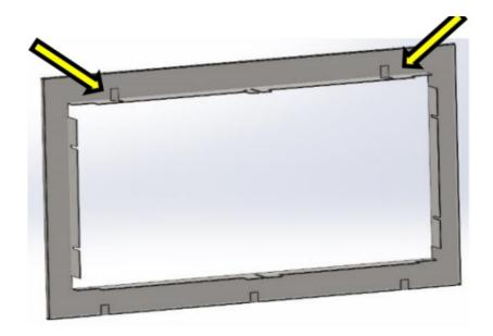
3. BEND THE SILICONE TABS INTO POSITION. THIS TAB SHOULD BE PARALLEL TO THE FRONT OF THE FASCIA WHEN IN THE CORRECT POSITION.
