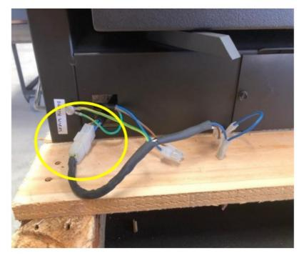
4. PLUG THE FAN SWITCH WIRING LOOM CONNECTOR TO THE FAN CONNECTOR
