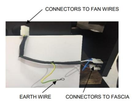
2. UNPLUG THE FAN CONNECTOR FROM THE FASCIA CONNECTOR, UNSCREW
