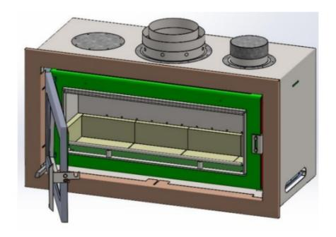
5. RE INSTALL THE DOOR BACK ON. USE THE REVERSE METHOD TO REMOVAL ON POINT 1.
