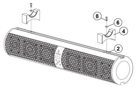
2. Secure bracket [4] to slider [2] with short bolt [6] and washer [8].
