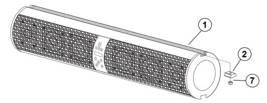
Put the nut [7] into the lower slot of the slider [2], and push the slider [2] onto the slide rail of the speaker.
