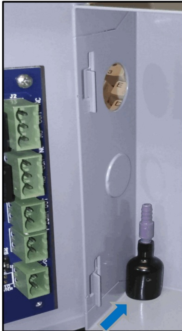
Figure 10: Oxygen sensor calibration cap, stored in the lower right of the enclosure
