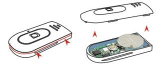
2. After replacing the battery, reverse assembly.
