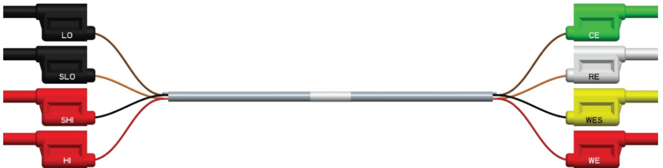
Figure 9: Four-electrode cell testing cable connections
