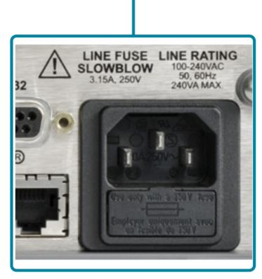
3. Connect the plug of the power cord to a grounded AC outlet.
