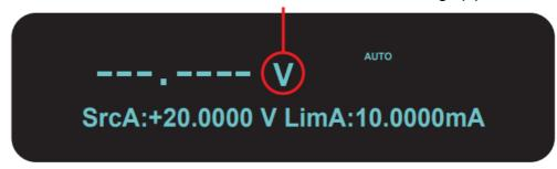
2. Press the **AUTO** key as many times as needed to select the AUTO range function. When AUTO is selected, the 2601B- PULSE automatically selects the best range for the measured value. You will briefly see the display shown below, and then the main display screen reappears.
