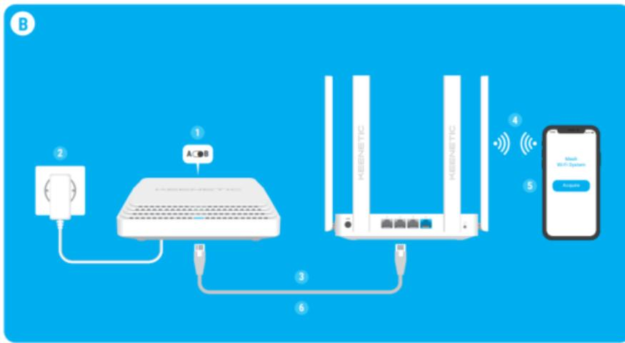
1. On the Keenetic device you wish to be a Mesh Wi-Fi Extender, set the **Operating Mode Switch** located on the back panel to position
